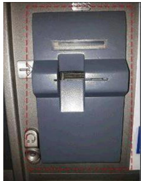
An unusual card reader installed at the card slot
